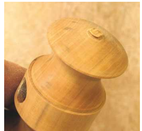
▲ Pic.27 When cutting off the waste make sure that you leave a little extra on top rather than cutting it off flat, to allow you to dome it over with the sandpaper
